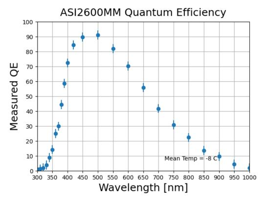
Figure 2. Measures camera quantum efficiency uncorrected for camera window transmission. Absolute calibration may be off due to exact sensor placement.
