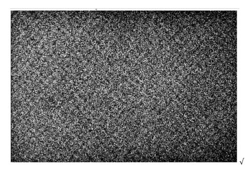
Figure 3. Median combined flat field image at 320 nm.
